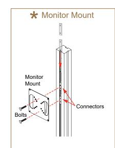
Slide connectors into groove of extrusion. Tighten set screws to secure connectors in place. Attach monitor mount back plate to extrusion, using bolts.
