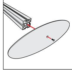
**Base Plate & Extrusion Connection**
