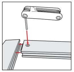
**Extrusion & Lock Connection**
