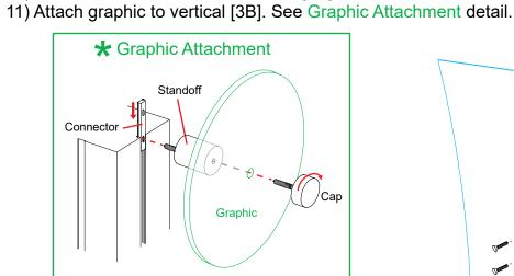
Slide connector into groove of vertical extrusion. Tighten set screws to secure in place. Screw standoff into connector. Place graphic between standoff and cap then screw cap to tighten in place.
